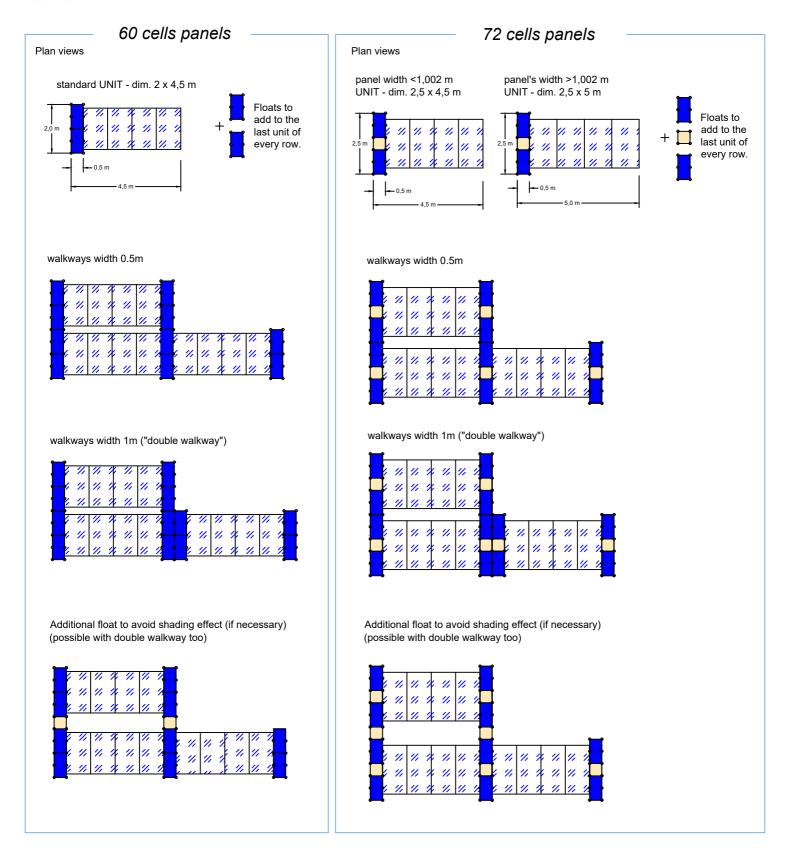
For every layout case it is possible to add extra walkways to enlarge the passage, even in the horizontal direction.
